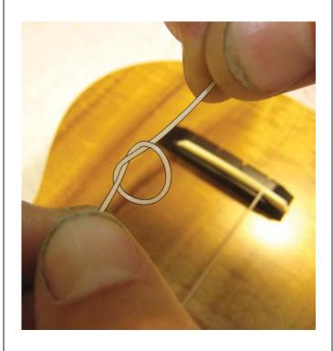
Full the knot tight and clip the excess string about 1/8" from the knot.
